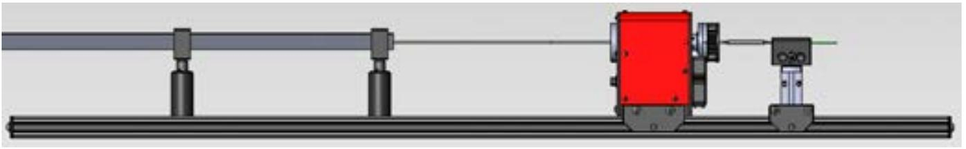
CONFIG #2: Spindle on the left side, clamp on the right side. Recommended to use with catheters with short to medium length balloons and non-circular shaft tubing. Recommend to use segmented or touhy borst chucks on the spindle. The chuck will hold the proximal side of the balloon and rotate. Clamp will hold the distal end of the support mandrel.
