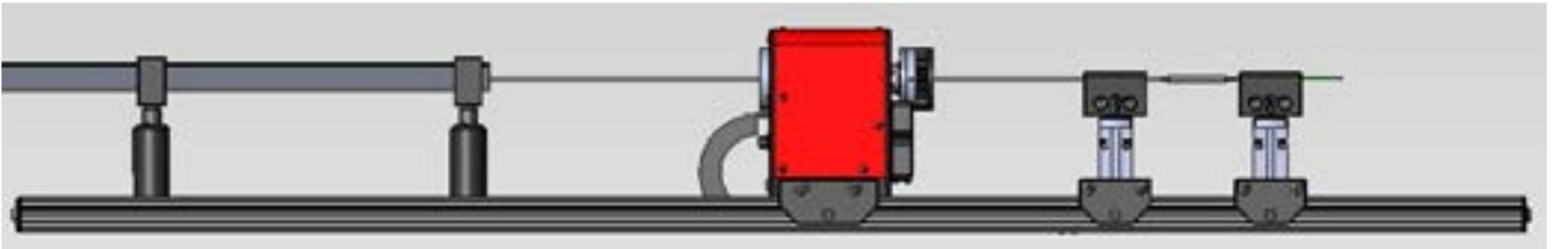
CONFIG #3: Spindle on the left side, dual clamps on each side of the balloon. Recommended to use with catheters with short to long length balloons and long shaft. Recommend to use the segmented or touhy borst chucks on the spindle. The chuck will hold the proximal end of the catheter. Clamps will hold both proximal and distal end of the balloon. Allow drop-in loading, efficient and precise
