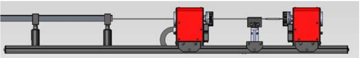
CONFIG #4: Dual spindle for holding catheters with built in guide wire or without through inner lumen, or for long and large size catheters
