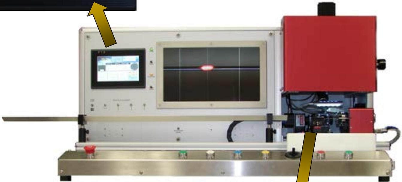
The new configurable drop loading catheter holding system allows fast loading/unloading. Right chuck can be a segmented chuck with 0-1/4" opening, touhy borst or three jaw micro chuck. Air driven adjustable opening catheter clamp on the left. See other configurations on separate page. Adjustable position catheter support trough is standard.
