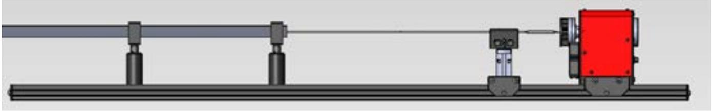
CONFIG #1: Spindle on the right side, clamp on the left side. Recommended to use with catheters with short to medium length balloons. Any types of chuck can be installed on the spindle. The chuck will hold the distal end of the support mandrel and rotate. Clamp will hold the proximal side of the balloon as a guide. Allow quick drop loading.
